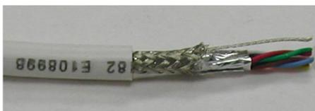
Predator Grizzly Cables have four layers of shielding. First, each wire is individually shielded with a polypropylene jacket. Second, an aluminum foil shield wraps around all of the pairs. Third, a metal braid shield is wrapped around the foil. Finally, a thick but flexible PVC jacket is wrapped around the metal braid. The quality and strength of the shielding included with Predator Grizzly cable protects your data from RF noise and electrical interferences.
